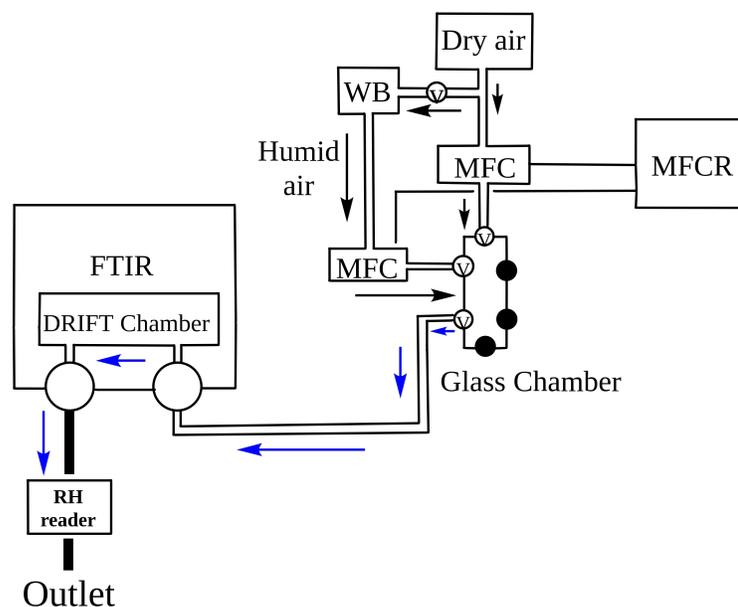
**Figure 4.** Schematic representation of the DRIFT apparatus and gas handling system. TC is thermocouple, RH refers to relative humidity, V refers to valves, MFC is mass flow controller, MFCR means readout for the mass flow controllers and WB is the water bubbler.
