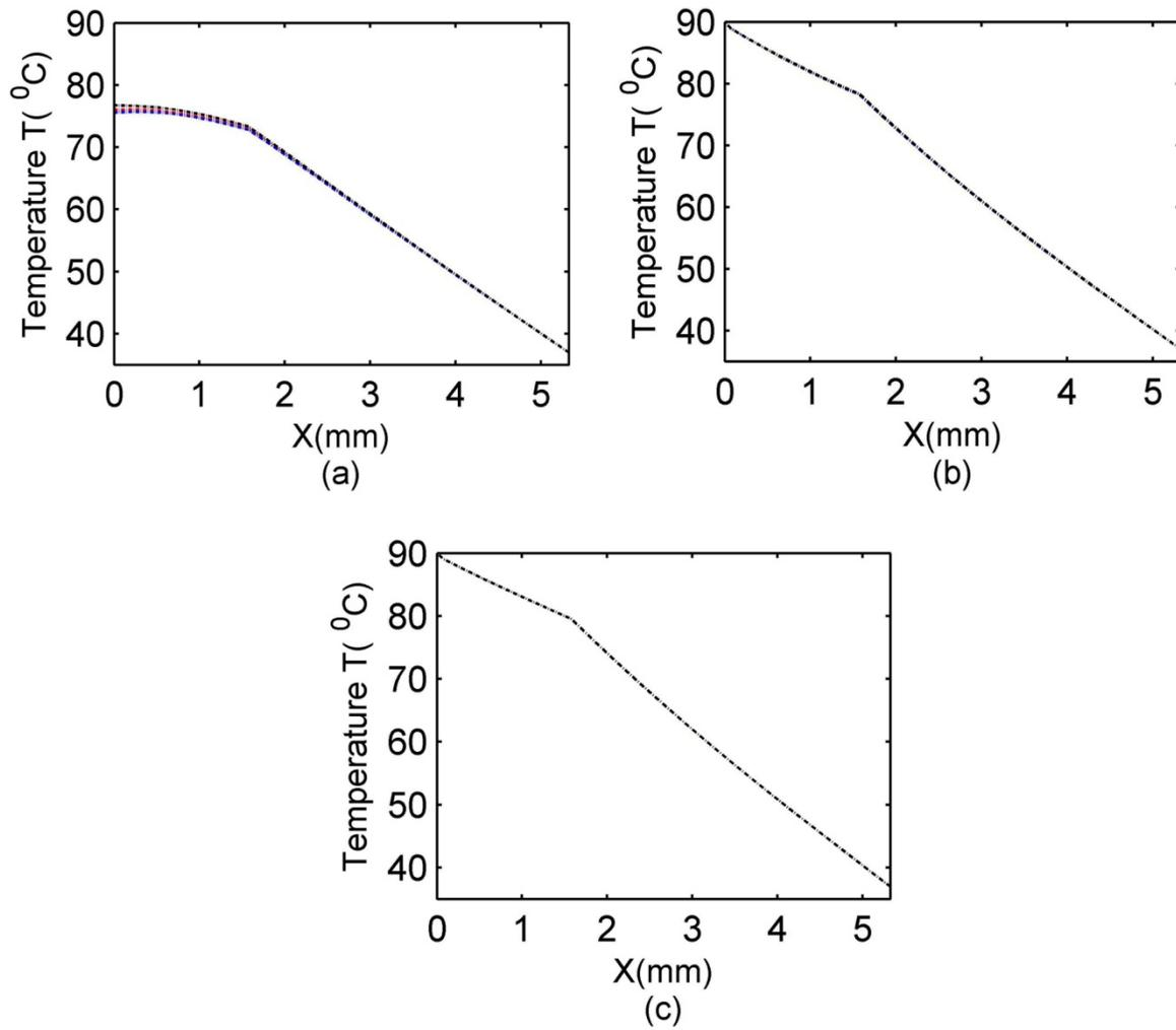
**Fig. 14** Effect of ambient temperature. (a)  $y = 0$  mm, (b)  $y = 3$  mm and (c)  $y = 7$  mm. Red lines,  $T_0 = 25^{\circ}\text{C}$ ; Black lines,  $T_0 = 40^{\circ}\text{C}$ ; and Blue lines  $T_0 = 16^{\circ}\text{C}$ .
