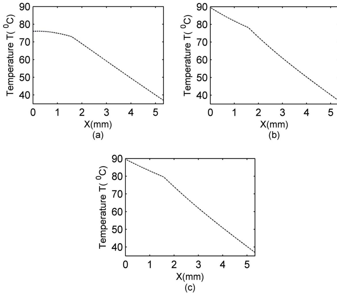
**Fig. 15 Effect of evaporation rate. (a)  $y = 0$  mm, (b)  $y = 3$  mm and (c)  $y = 7$  mm. Red lines,  $E = 10 \text{ Wm}^{-2}$ , Black Lines,  $E = 15 \text{ Wm}^{-2}$  and Blue lines,  $E = 0 \text{ Wm}^{-2}$ .**
