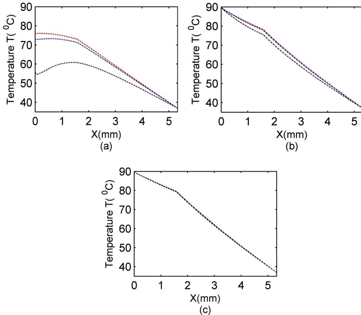
**Fig. 13** Effect of ambient convection coefficient. (a)  $y = 0$  mm, (b)  $y = 3$  mm and (c)  $y = 7$  mm. Red lines,  $h = 7 \text{ Wm}^{-2} \text{ K}^{-1}$ ; Black lines,  $h = 250 \text{ Wm}^{-2} \text{ K}^{-1}$ ; and Blue lines,  $h = 25 \text{ Wm}^{-2} \text{ K}^{-1}$ .
