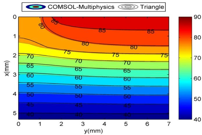
Fig. 3 Comparison results of triangle and COMSOL- Multiphysics.
