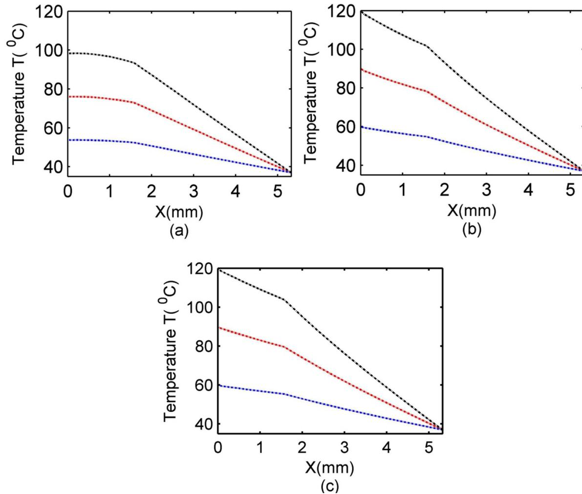
**Fig. 11 Effect of disk temperature. (a)  $y = 0$  mm, (b)  $y = 3$  mm and (c)  $y = 7$  mm. Red lines,  $T_d = 90^\circ\text{C}$ ; Black lines,  $T_d = 120^\circ\text{C}$ ; and Blue lines,  $T_d = 60^\circ\text{C}$ .**
