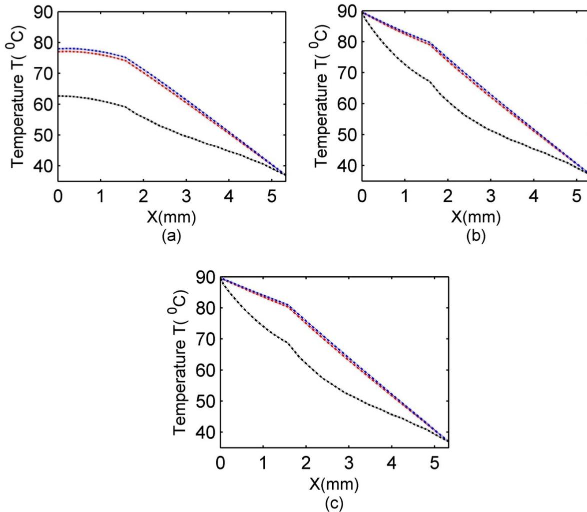
**Fig. 12 Effect of blood perfusion rate. (a)  $y = 0$  mm, (b)  $y = 3$  mm and (c)  $y = 7$  mm. Red lines,  $w_b = 0.00125$  ml/s/ml; Black lines,  $w_b = 0.024$  ml/s/ml; and Blue lines,  $w_b = 0.0005$  ml/s/ml.**
